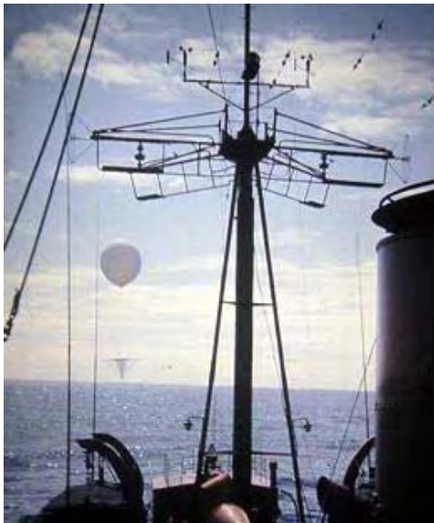
Figs 5 & 6: A helium filled balloon ready to launch with radar reflector – right, climbing skywards
